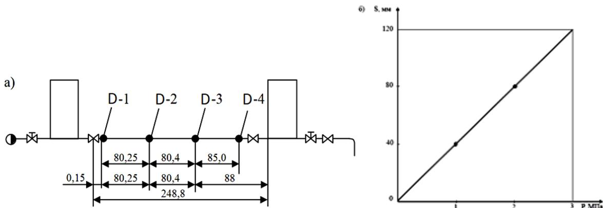
**Fig.2.** The arrangement diagram of the DD-10 (D-1,2,3,4) pressure sensors on the pressure pipeline (a) and the calibration graph of the DD-10 pressure sensor (D-1,  $P_c=23.0$ , No. P0962) using the N043.1 oscilloscope (b)
