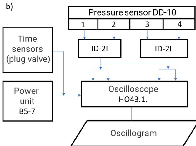
**Fig.1(b).** Block diagram of connection of control and measuring equipment.
