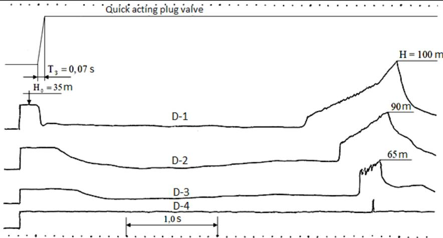
**Fig.4. Water hammer oscillogram (Experience 339,  $\vartheta_0=1,5$  m/s;  $H_g=15$  m,  $\varphi=0,01$ ).**
