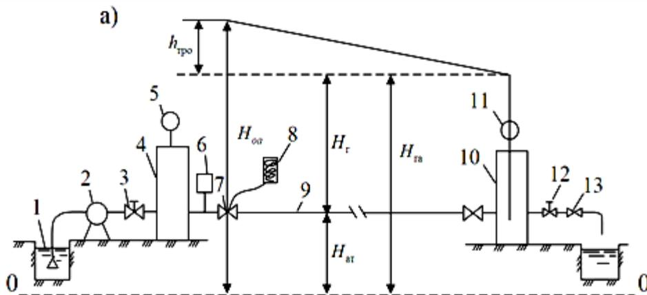
**Fig.1 (a). Scheme of the experimental setup:** 1- hydrometric tray; 2- centrifugal pump brand 4K-6; 3,12-valves; 4,10-pressure tanks; 5,11-standard pressure gauges; 6-compressed air supply unit; 7,13- quick acting plug valves; 8-solenoid brand KMP-4AUZ; 9- pressure pipeline.
