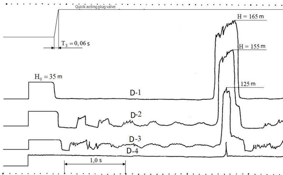
Fig.3. Water hammer oscillogram (Experience 333,  $v_0=1,5$  m/s;  $H_g=15$  m,  $\varphi=0$ ).
